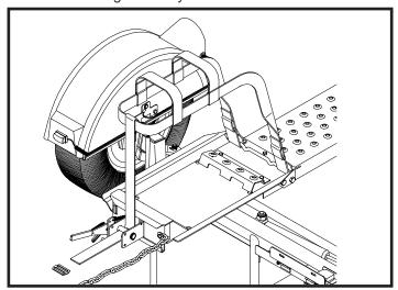
Step 8. Place one tie-down strap over each tire and secure hooks to rods located at the rear of each wheel platform. The short side of the hook must face the rear of the Kar Kaddy.
